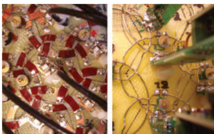
The radio-frequency coils used to transmit and detect MRI signals are being made more sensitive.
